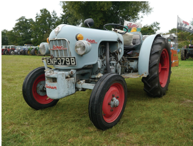
1956 Eicher. West German built, 2-cylinder, air cooled tractor.
