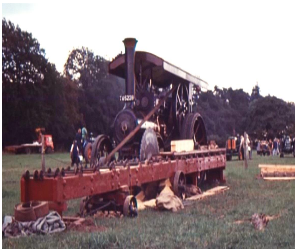
Burrell Steam engine driving the saw bench, previously owned by John Bourne
