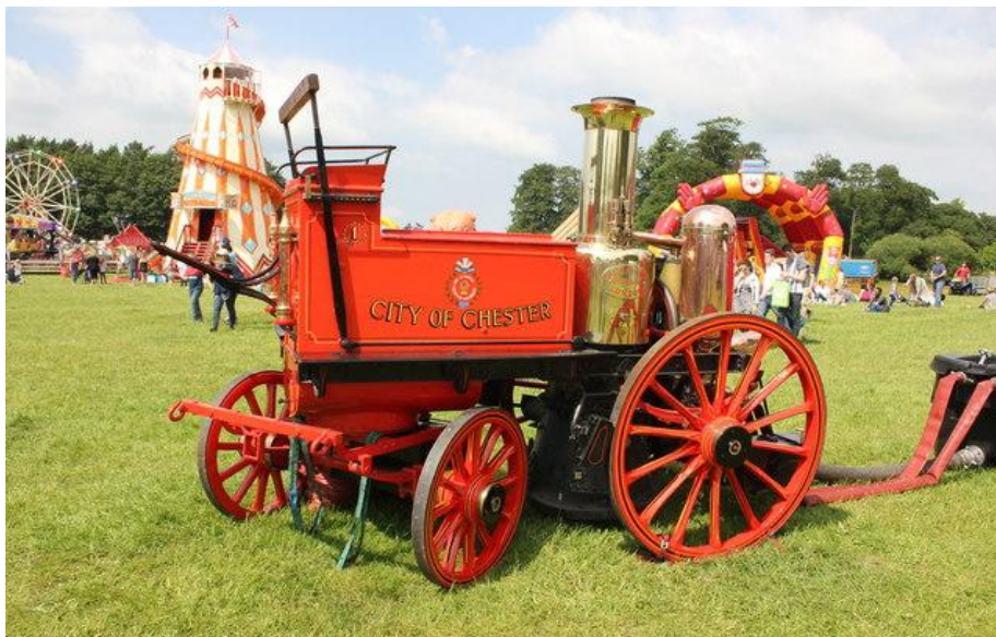
Ex City of Chester Steam actuated Fire Pump
